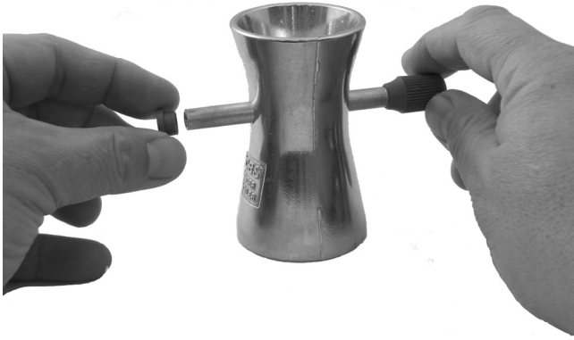
Photo 3 Insert tube and install retaining ring
