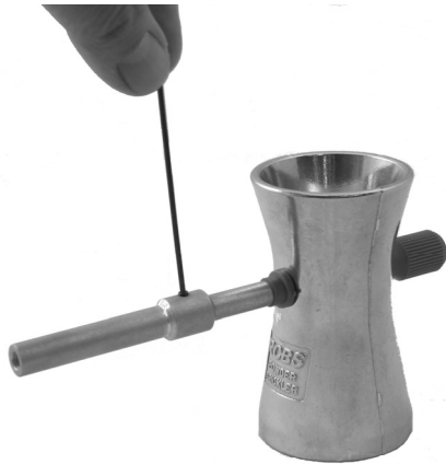
Photo 4 Secure extension tube set screw
